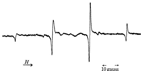
Fig. 4. ESR spectrum of the methyl radical on the silica gel surface at 77°K. The silica gel was pretreated by evacuating for 15 hr without heating.
